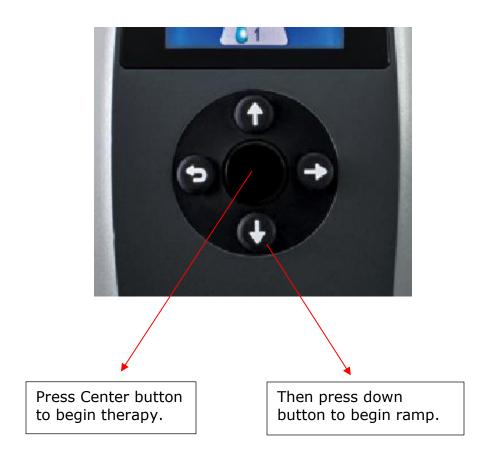
**Note:** If the miniCPAP<sup>™</sup> device loses power while delivering therapy, the CPAP will power on as soon as power is restored. The user must hit the Center button to resume therapy.
