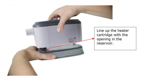
5. Once the reservoir is filled completely, set it on a secure, flat surface and line up the CPAP heater cartridge with the opening in the reservoir. Hold the reservoir in place and set the CPAP onto it so that the magnets snap the pieces together securely.
